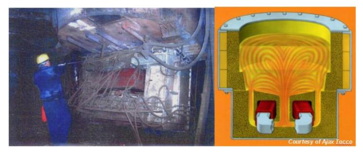
Severe Restriction of Metal Flow in Throats or Inductor Channels can caused heavy saturation leading to refractory wear or metal leakage. Inability to superheat the molten iron.
