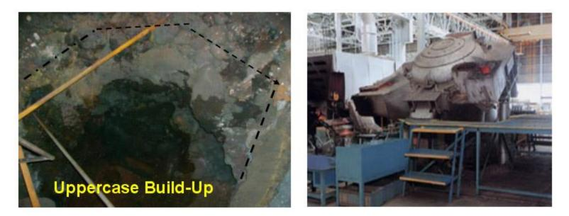
Furnace history will indicate when to flux. Establish the "threshold" indicator such as a minimum/maximum limit to conductance /reactance depending on equipment.
