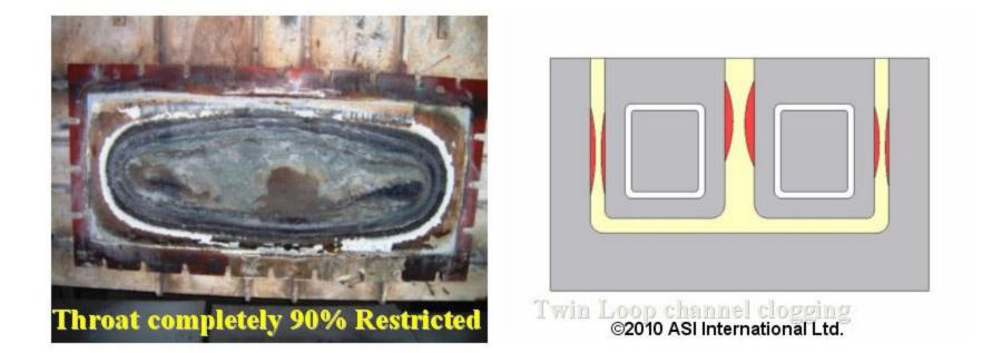
In 48 hrs, foundry experienced severe Build-Up in throat and each of the channels of a Double-loop inductor.
